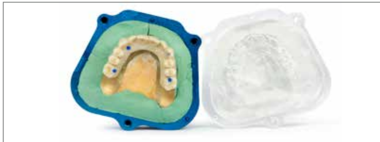
Place the model back in the flask, close the screwholes with teflon and wax and carefully screw the top part back on the flask. Check perfect positioning.
