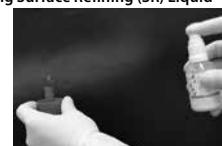
Spray just once (1x) on the internal / external surface of the wax pattern. Keep a distance of 15cm for an optimal dispersion of the spray.
