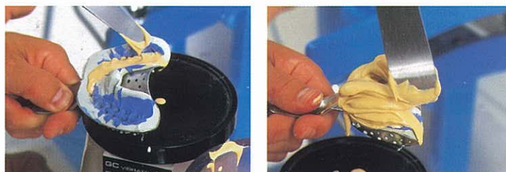
Free-flowing consistency, despite thixotropic properties
